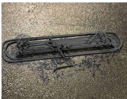
Figure 7.13: First try to print bending part with Ti6:PEG:PVB:SA 3 vol.% feedstock
