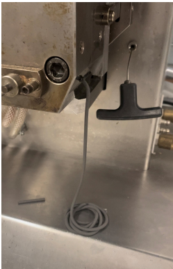
Figure 7.30: Extruded filament of F3SA3MC presenting good extrudability
