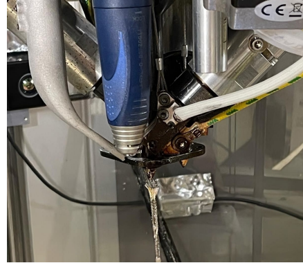
(b) Thermocouple inserted in a 1 mm brass nozzle
