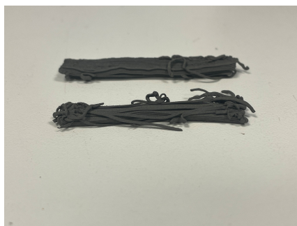
Figure 7.14: Printing test of TiPEGPVBSA with 3 vol.% of SA
