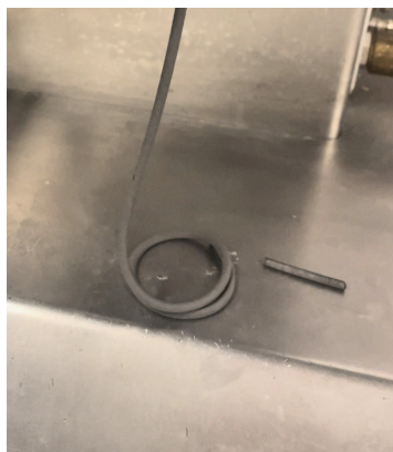
(b) PolyMIM at 180°C and 60 RPM: filament retains its shape.
