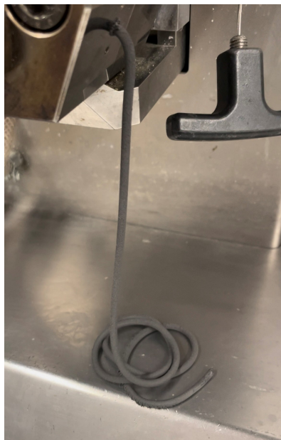
Figure 7.18: Extruded filament with 3 vol.% of MC
