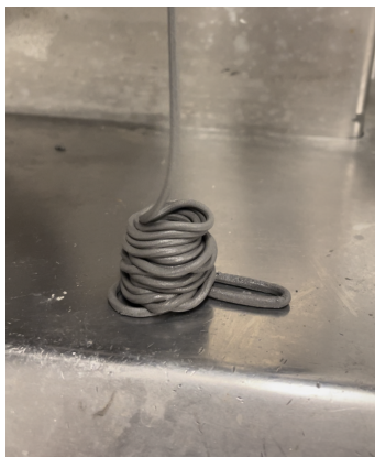
(a) F5SA at 110°C and 60 RPM: filament deforms under its own weight.
