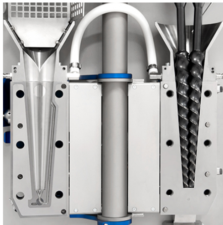
Figure 5.5: Xplore DSM twin screws micro-compounder MC 15EHT [215]
